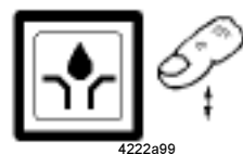
Fig. 21 - Pushbutton for additional lubrication cycle
