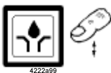
Fig. 31 - Push button for an additional lubrication cycle
