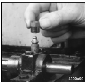
Fig. 5 - Place the Zerk-Lock body over the grease fitting
