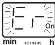
Fig. 22 - Display of a fault indication
