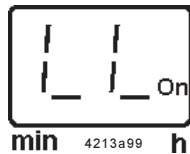
Fig. 26 - Display for an acknowledged low level control
