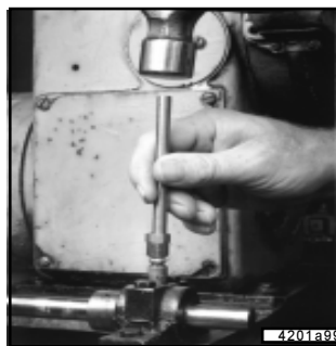
Fig. 6 - Installation of Zerk-Lock body with staking tool
