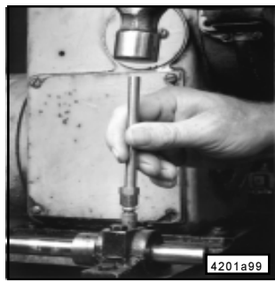
Fig. 6 - Installation of Zerk-Lock body with staking tool
