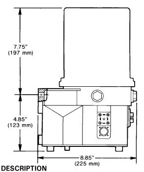
The lube pump is electrically operated and used in a progressive type centralized lubrication system. The pump consists of a pump housing, electric gear motor and a plastic reservoir with stirring paddle. The high operating pressure allows the pump to supply lubricant up to NLGI 2 grease.
