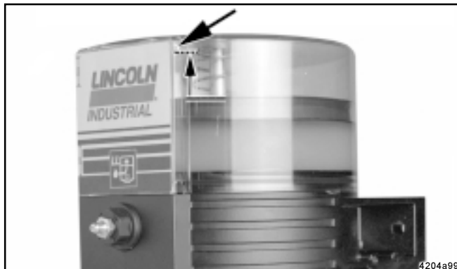
Fig. 11 - Vent hole on reservoir
