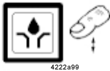
Fig. 22 - Pushbutton for additional lubrication cycle
