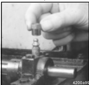
Fig. 6 - Place the Zerk-Lock body over the grease fitting
