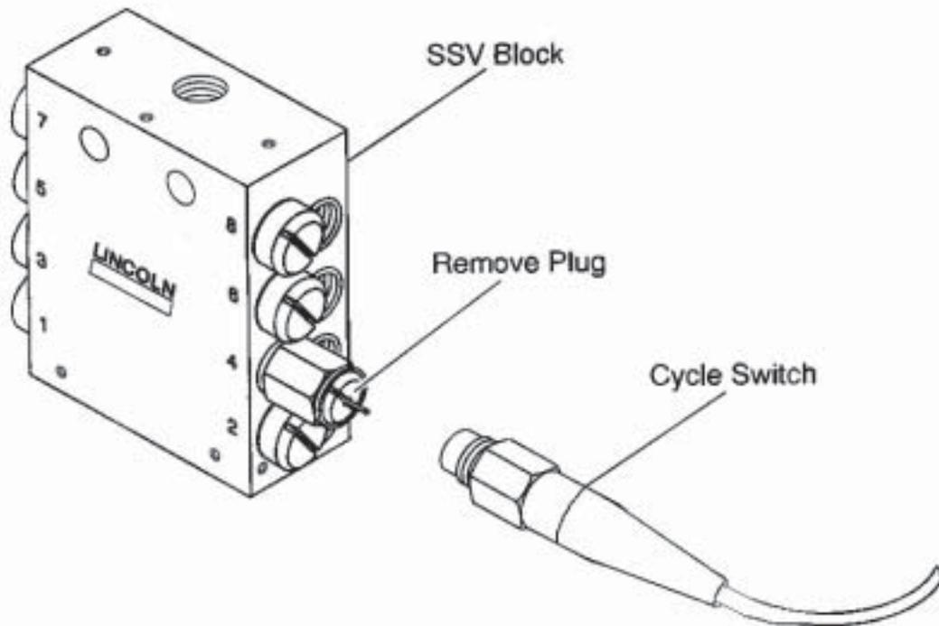
**DESCRIPTION:** Cycle switch can provide feedback monitoring for SSV systems.
